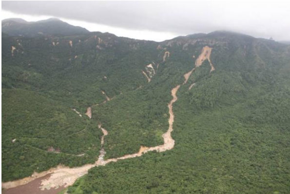
Fig. 8 Mobile debris flows on Lantau in the June 2008 rainstorm
